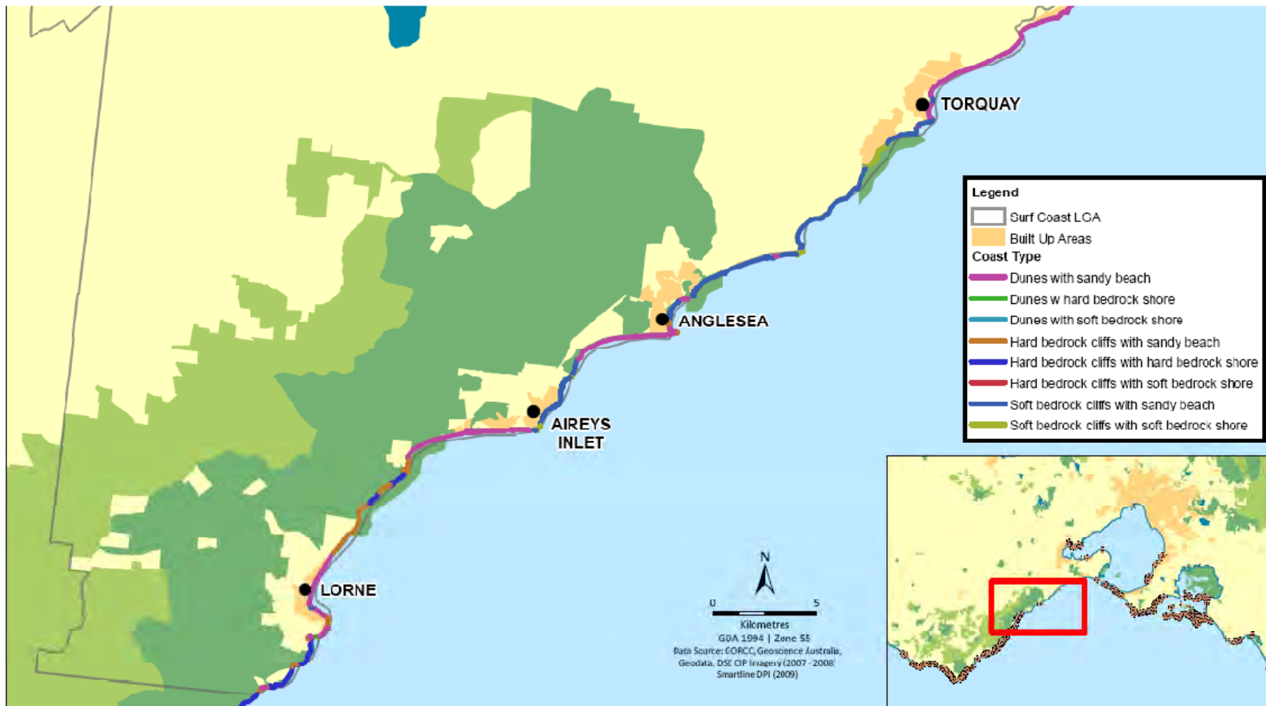
Figure 4 Coastal landforms of the Surf Coast region. Coastal areas that were assumed to be resistant to erosion and recession were those with hard rock cliffs, with either sandy or rocky shorelines. Coasts with sandy shorelines in front of hard rocky cliffs would be vulnerable to erosion, but are unlikely to recede. Data derived from [17].
